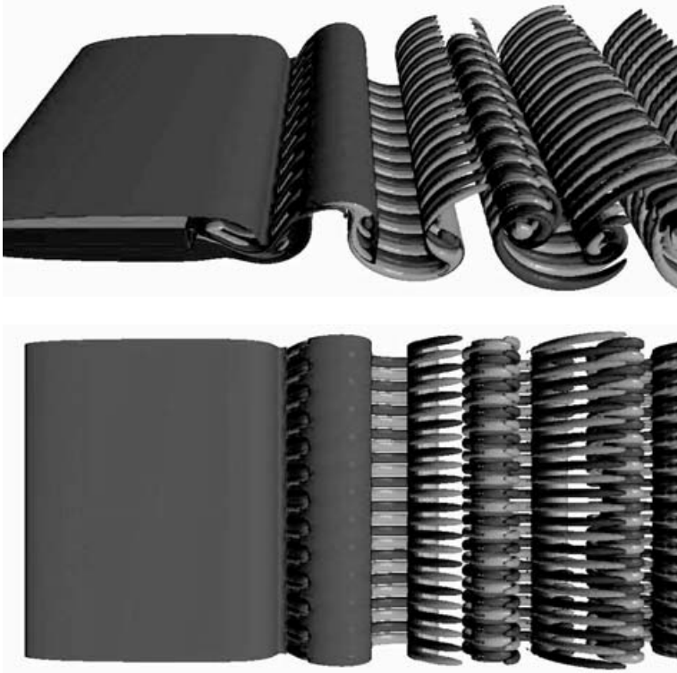
FIGURE 19. Isosurfaces of the streamwise vorticity field for the Floquet Mode C. Isosurfaces of spanwise vorticity ( \omega_z = \pm 0.5 ) are also shown to show the positions of the Kármán vortices. Spanwise wavelength is 1H and 12 wavelengths are shown. ( Re = 400 , AR = 7.5 ).
